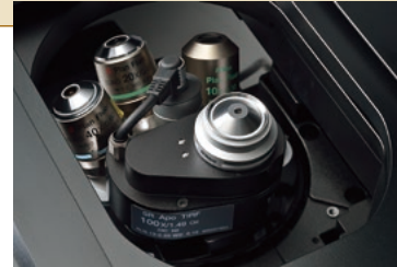
CFI SR HP Apochromat TIRF 100XC Oil CFI SR Plan Apochromat IR 60XC WI
